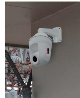
Ganz PT Thermal Camera mounted on a Standard Wall Bracket (WMK3-1W).
