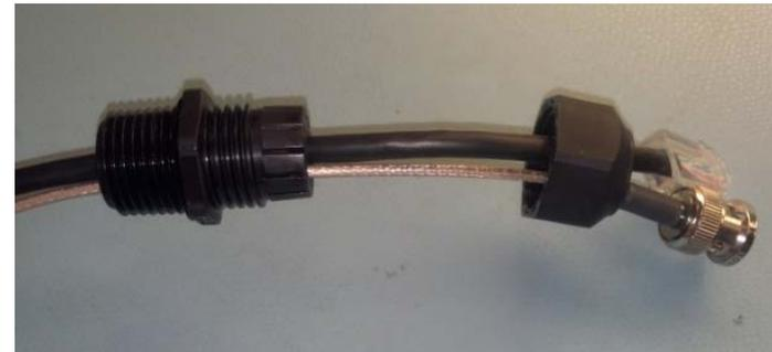
4. Tighten the gland nut onto the gland housing. Leave about 5 inches of cable sticking out of the gland housing
