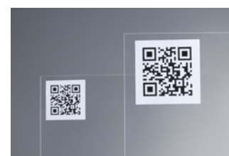
Image captured with RICOH Extended Depth of Field Camera QR codes in foreground and background are both readable.
