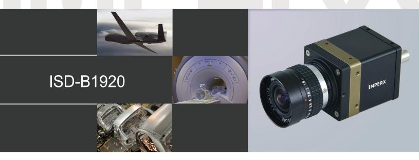
IMPERX ISD-B1920 is an advanced progressive scan, fully programmable CCD camera designed for imaging applications that require high quality images, powerful features and flexibility. The camera is small, light weight, and built around Kodak's KAI-2093 7.4 micron Interline Transfer CCD image sensor with a 1" optical format.
