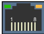
8-pin RJ45 jack connector with 2 built-in LED indicators
