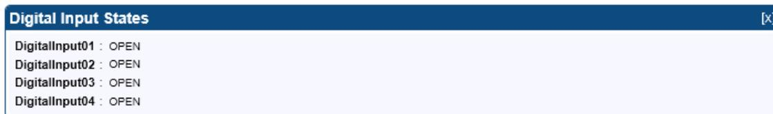
The Digital Input States are refreshed automatically every 2.5 seconds.
