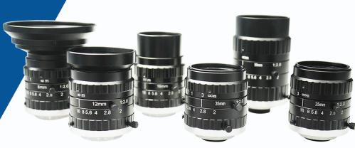
AZURE has released a new lens series for 2/3" sensors (image circle maximum to 13.4mm). The new M6M series is optimized for close working system: 0.2 - 0.4 m. The presented products are 6 megapixel, fixed focal length models dedicated to sensors with a pixel size down to 3 µm. Coating of new lenses produces a high transmission in 400-950 nm spectral range. The offer includes lenses with focal lengths: 8mm, 12mm, 16mm, 25mm, 35mm and 50mm.
