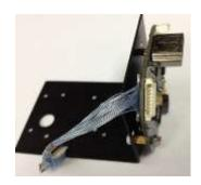
The Micro-coaxial cable is already attached to the interface board and the user can connect the other end to the Sony camera as illustrated.
