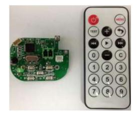
Power is connected via a 2position screw terminal block on the control board (green connector) at 12VDC.
