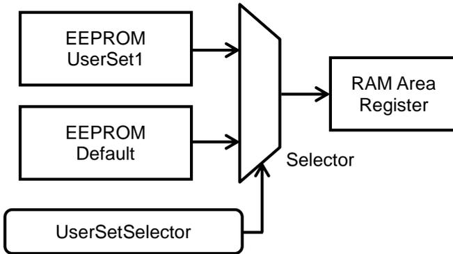
When executing UserSetLoad, write the camera setting information from the RAM into the memory area that was selected on the UserSetSelector.
