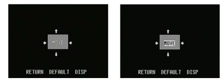
Move the cursor to the desired location and press the E button. Then the blinking cursor turns solid (black) and, in the example shown in the above figure, you can use the U, D, L, and R buttons to move the MOVE position to the desired location. To change the size, use the U and D or L and R buttons. To change the desired location, press the E button and the blinking solid (black) cursor changes to a normal blinking cursor, enabling you to move it using the U, D, L, and R buttons.
