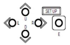
Hold down the menu button for longer than 2 seconds to display the main menu. Through this menu, you can set up camera functions. You can select any of the blinking items. To move to the next page, select PAGE and press the R button. To go back to the previous page, press the L button.
