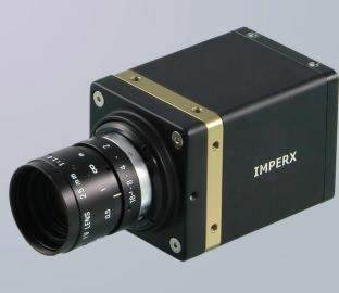
The IGV-B1410 is an advanced progressive scan, fully programmable CCD camera designed for imaging applications that require high quality images, powerful features and flexibility. The camera is small, weight, and built around SONY's ICX-285 6.45 micron Interline Transfer CCD image sensor with a 2/3" optical format.
