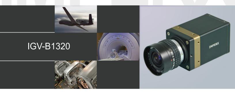
The IGV-B1320 is an advanced progressive scan, fully programmable CCD camera designed for imaging applications that require high quality images, powerful features and flexibility. The camera is small, light weight, and built around Kodak's KAI-01150 5.5 micron Interline Transfer CCD image sensor with a 1/2" optical format.
