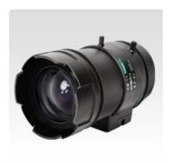
High image-quality monitoring with optical performance supporting 5 megapixels. Advanced design engineering and special optic glass adopted, best suited for color, Black & White, and Day and Night cameras. f12.5-50mm, 4x zooming application compatible lens. Designed to maximize optical performance with high-accuracy aspheric lens, low-dispersion glass, and high refractive-index glass. Built-in ND filter of T360, supporting high sensitivity cameras.
